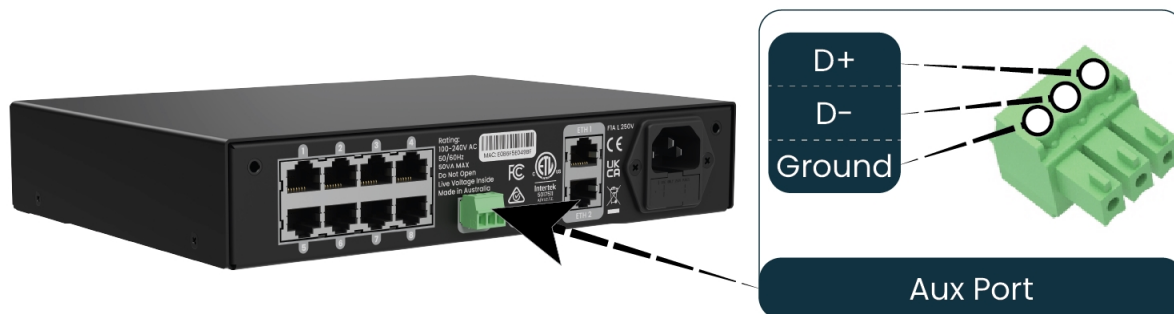
Figure 20: Location and Pinout of the Aux Port
