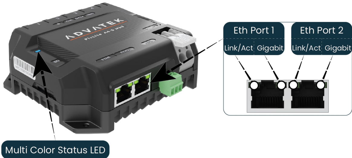
Figure 16: Location of LEDs
