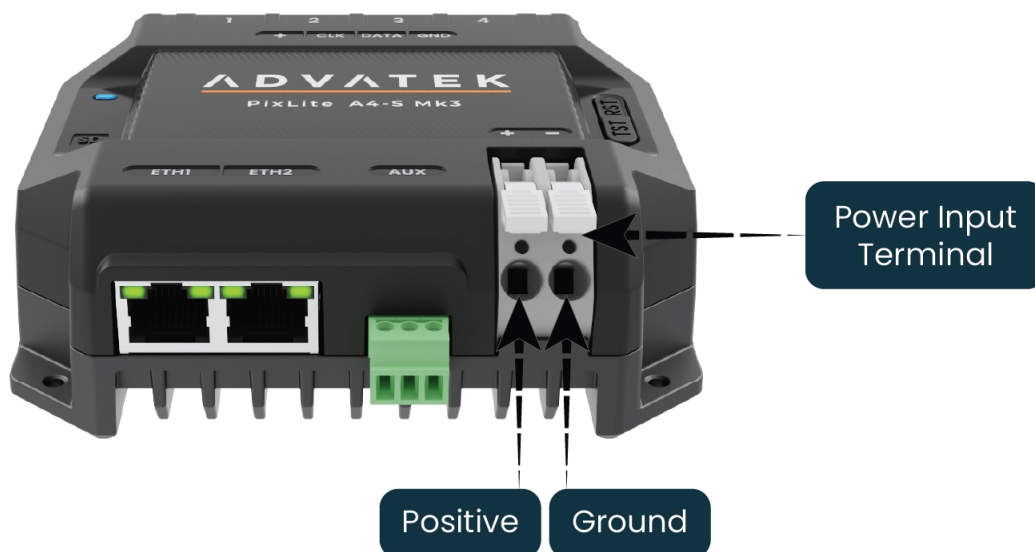
Figure 6: Location of Power Input
