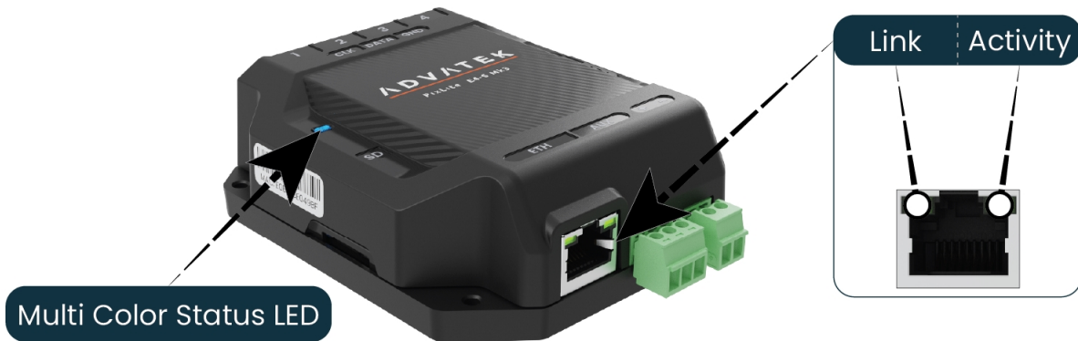
Figure 15: Location of LEDs
