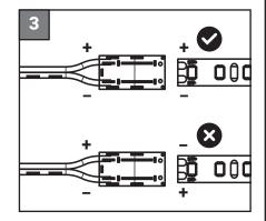
3. Insert strip light into the solderless connector and check the polarity.
