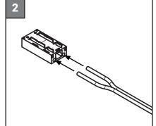
2. Insert wires into the solderless connector.
