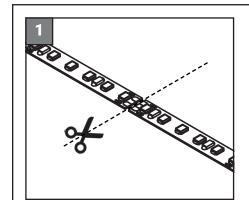
1. Cut the strip light at your desired length using the marked cut-points.
