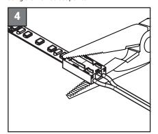
4. Compress the metal clips on the solderless connector to secure the wire and strip light.
