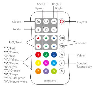
Mode+/-: Short press switch dynamic mode built in controller, long press 2s
