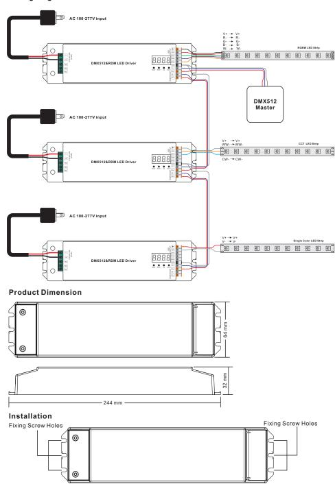
**Note**: when mounting the driver, please choose any one of the three fixing screw holes to fix with a screw at each end.
