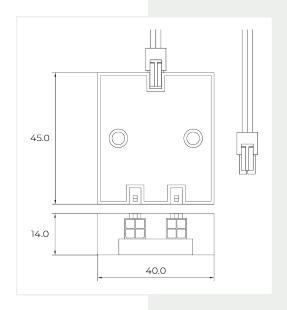
2 PORT SENSOR SPLITTER - WITH ACCESSORY PORT CONNECTION
